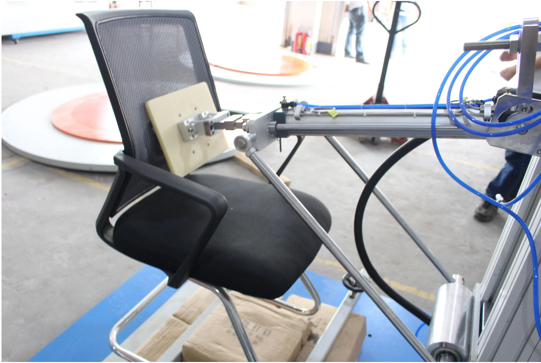
Office chair base vertical pressure testing setup with load application mechanism
